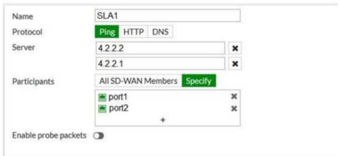
The screenshot shows the configuration for a performance SLA named 'SLA1'. The 'Protocol' is set to 'Ping'. The 'Server' field contains two entries: '4.2.2.2' and '4.2.2.1'. The 'Participants' field is set to 'All SD-WAN Members' with a 'Specify' button. Below this, two ports are listed: 'port1' and 'port2'. The 'Enable probe packets' checkbox is currently unchecked.
