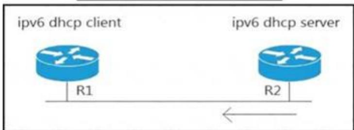
A network administrator is troubleshooting IPv6 address assignment for a DHCP client that is not getting an IPv6 address from the server. Which configuration retrieves the client IPv6 address from the DHCP server?
