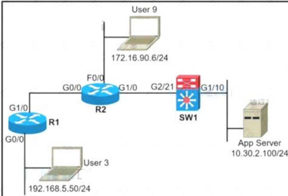
A network administrator must block ping from user 3 to the App Server only. An inbound standard access list is applied to R1 interface G0/0 to block ping. The network administrator was notified that user 3 cannot even ping user 9 anymore. Where must the access list be applied in the outgoing direction to resolve the issue?
