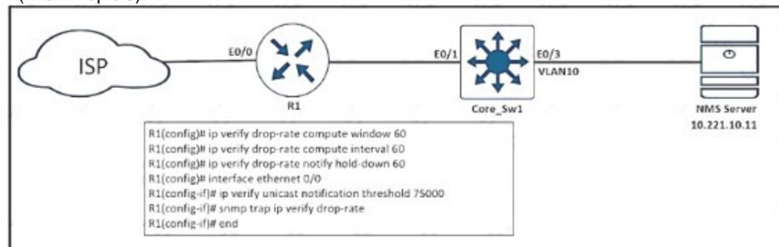
Refer to the exhibit. An engineer configured SNMP traps to record spoofed packets drop of more than 48000 a minute on the ethernet0/0 interlace. During an IP spoofing attack, the engineer noticed that no notifications have been received by the SNMP server. Which configuration resolves the issue on R1?
