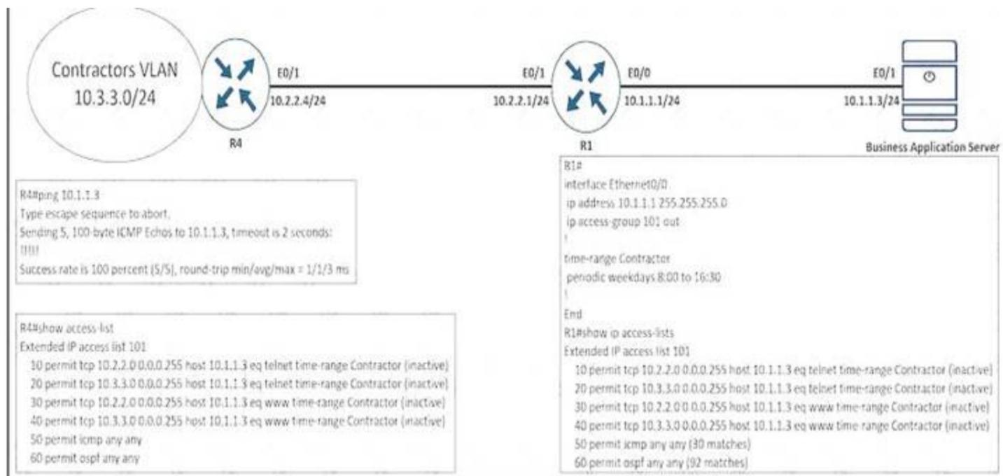
An engineer is troubleshooting failed access by contractors to the business application server via Telnet or HTTP during the weekend. Which configuration resolves the issue?
