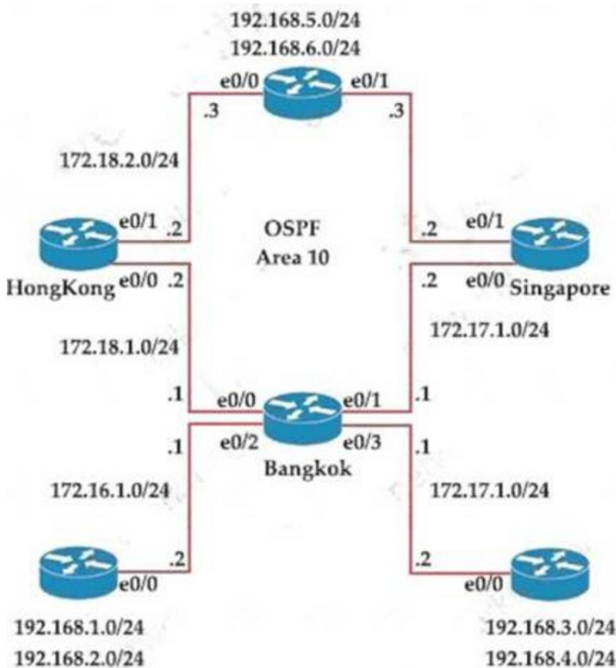
Bangkok is using ECMP to reach to the 192.168.5.0/24 network. The administrator must configure Bangkok in such a way that Telnet traffic from 192.168.3.0/24 and 192.168.4.0/24 networks uses the HongKong router as the preferred router. Which set of configurations accomplishes this task?
