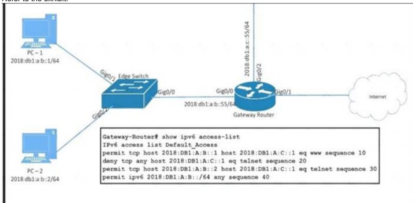
PC-2 failed to establish a Telnet connection to the terminal server. Which configuration resolves the issue?
