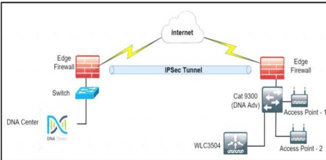
A network administrator is discovering a Cisco Catalyst 9300 and a Cisco WLC 3504 in Cisco DNA Center. The Catalyst 9300 is added successfully However the WLC is showing [ error "uncontactable" when the administrator tries to add it in Cisco DNA Center. Which action discovers WLC in Cisco DNA Center successfully?
