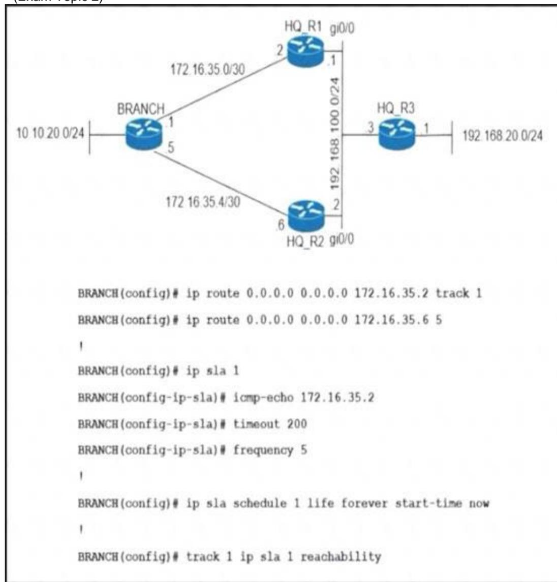
Refer to the exhibit. An engineer has successfully set up a floating static route from the BRANCH router to the HQ network using HQ\_R1 as the primary default gateway. When the g0/0 goes down on HQ\_R1, the branch network cannot reach the HQ network 192.168.20.0/24. Which set of configurations resolves the issue?
