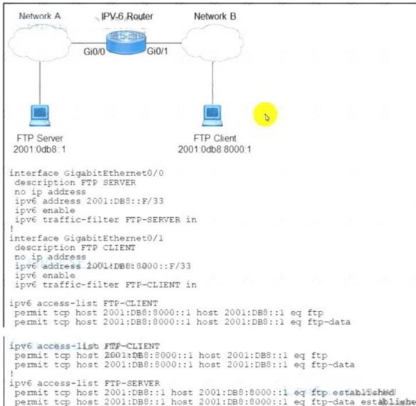
Refer to the exhibit. When an FTP client attempts to use passive FTP to connect to the FTP server, the file transfers fail Which action resolves the issue?
