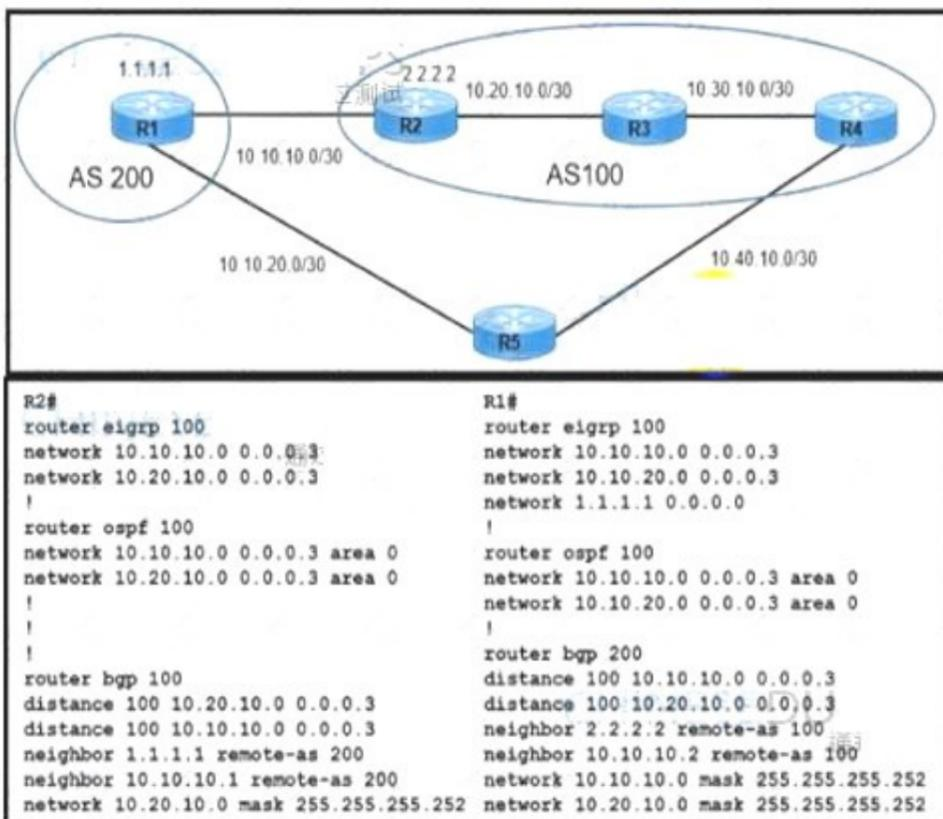
R1 and R2 use IGP protocol to route traffic between AS 100 and AS 200 despite being configured to use BGP. Which action resolves the issue and ensures the use of BGP?
