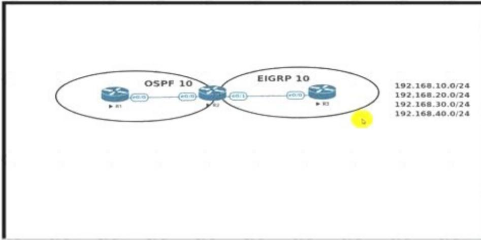
An engineer must redistribute networks 192.168.10.0/24 and 192.168.20.0/24 into OSPF from EIGRP. where the metric must be added when traversing through multiple hops to start an external route of 20 The engineer notices that the external metric is fixed and does not add at each hop. Which configuration resolves the issue?
