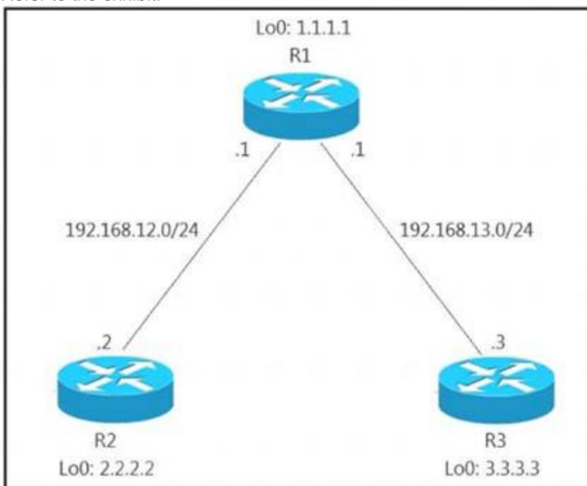
An engineer has configured R1 as EIGRP stub router. After the configuration, router R3 failed to reach to R2 loopback address.
