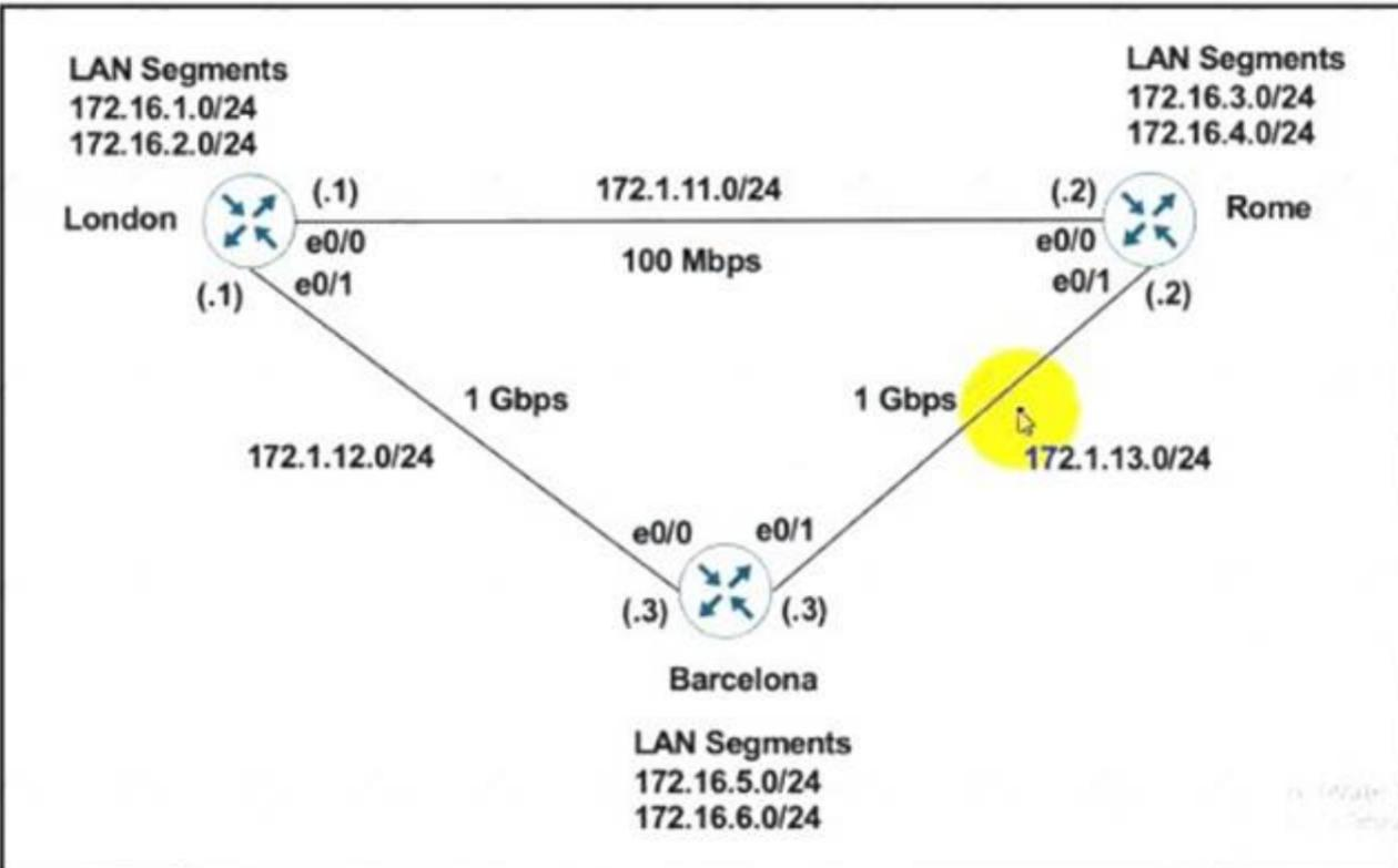
London must reach Rome using a faster path via EIGRP if all the links are up but it failed to take this path Which action resolves the issue?
