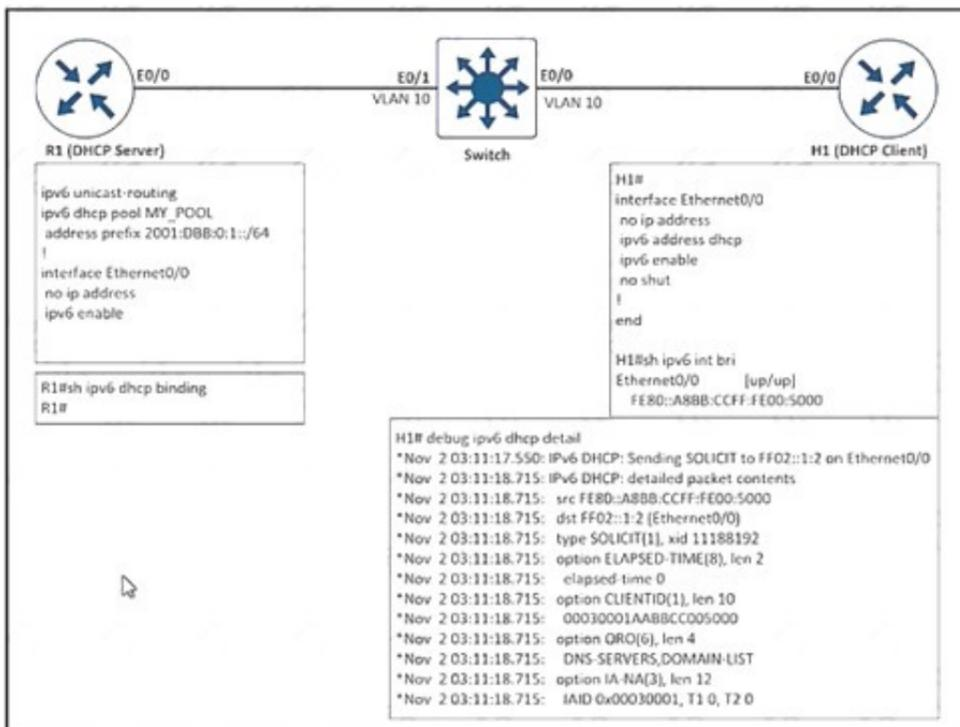
After the network administrator rebuilds the IPv6 DHCP server, clients are not getting the IPv6 address lease. Which action resolves the issue?
