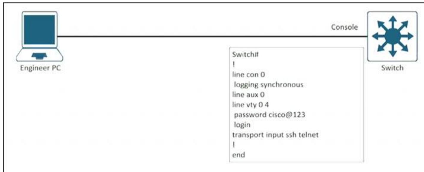
An engineer must block access to the console ports for all corporate remote Cisco devices based on the recent corporate security policy but the security team still can connect through the console port. Which configuration on the console port resolves the issue?
