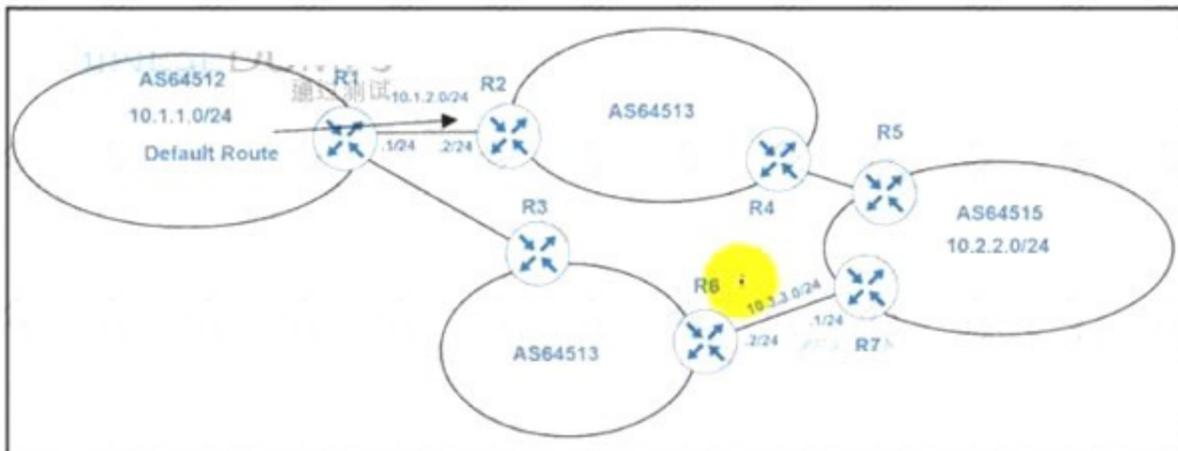
An engineer must configure PBR on R1 to reach to 10.2.2.0/24 via R3 AS64513 as the primary path and a backup route through default route via R2 AS64513. All BGP routes are in the routing table of R1, but a static default route overrides BGP routes. Which PBR configuration achieves the objective?
