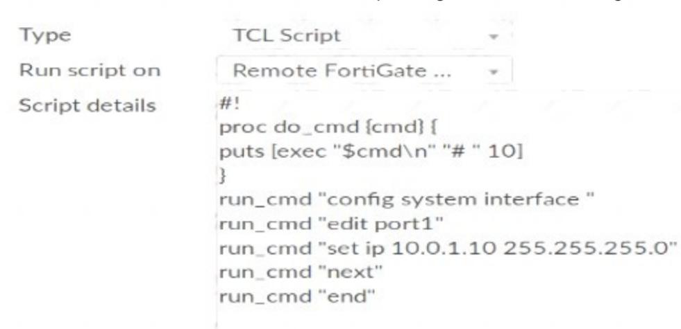
An administrator has configured the TCL script on FortiManager, but failed to apply any changes to the managed device after being executed.
