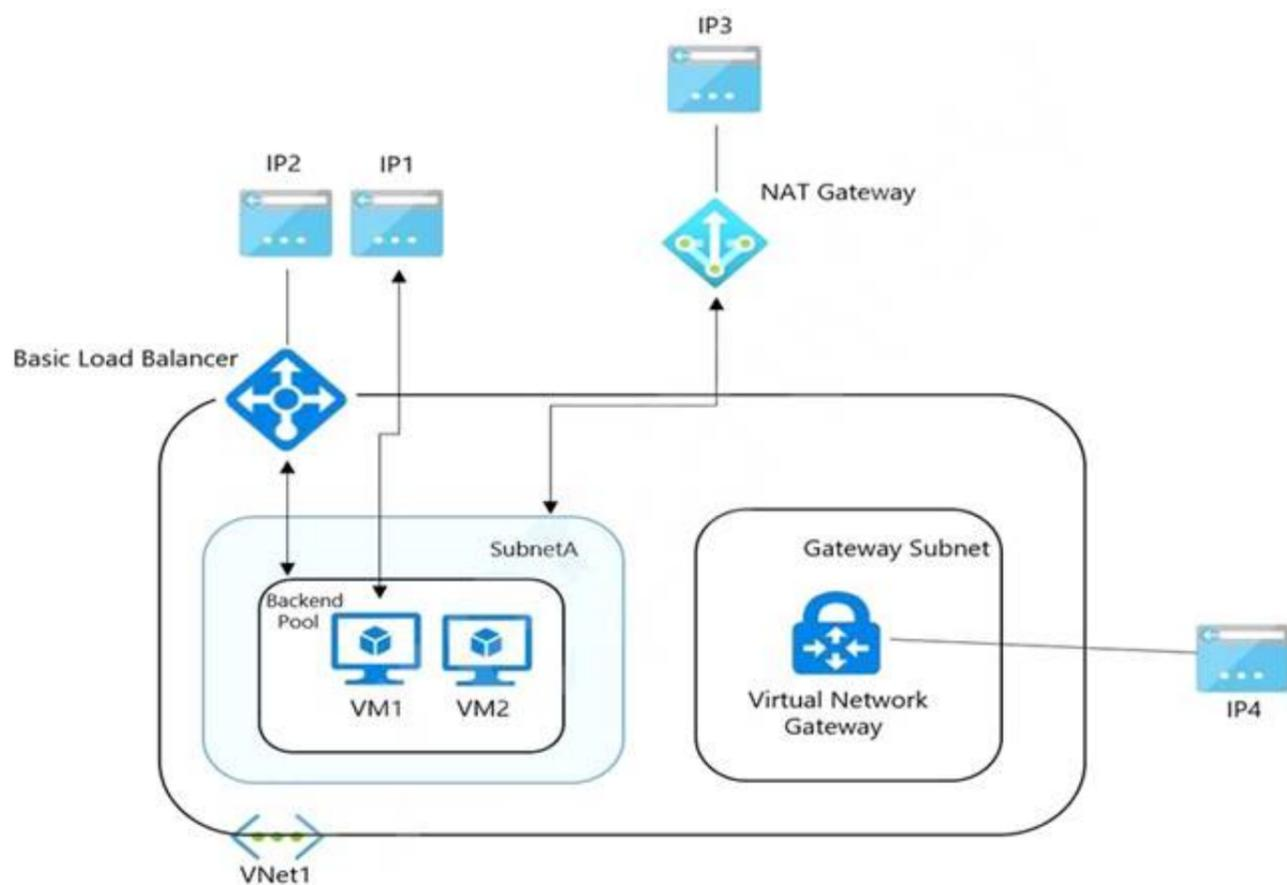
VM1 is a virtual machine that has an instance-level public IP address (ILPIP). Basic Load Balancer uses a public IP address. VM1 and VM2 are in the backend pool. NAT Gateway uses a public IP address named IP3 that is associated to SubnetA. VNet1 has a virtual network gateway that has a public IP address named IP4. When initiating outbound traffic to the internet from VM1, which public address is used?
