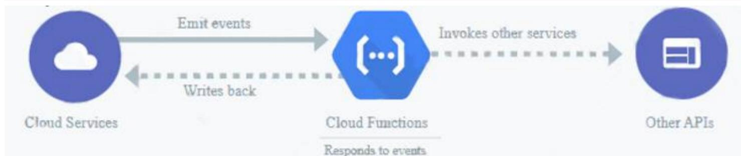
Cloud Functions is Google Cloud's event-driven serverless compute platform. It automatically scales based on the load and requires no additional configuration. You pay only for the resources used.
