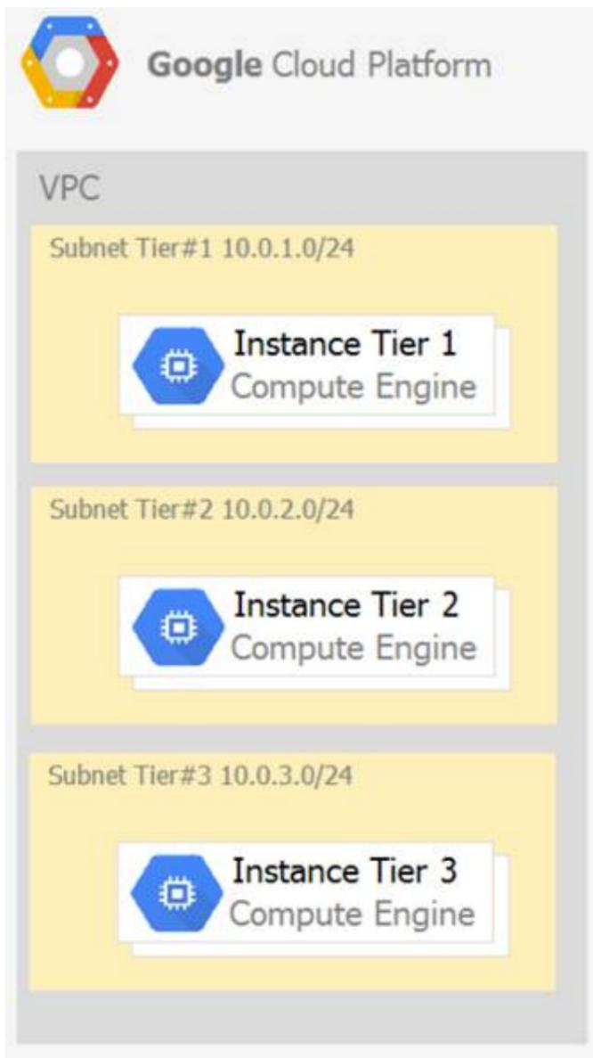
Each tier has a service account that is associated with all instances within it. You need to enable communication on TCP port 8080 between tiers as follows:
